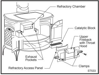
Fig. 32 Removing the catalytic element.
